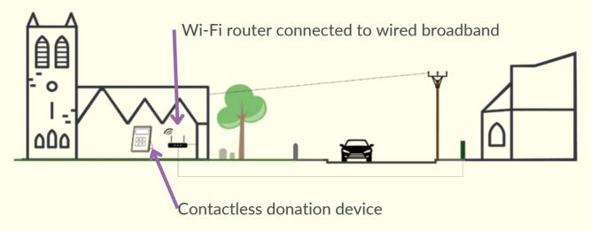
Broadband connectivity is where a cable is brought into the church building, either underground or overground. The cable would be connected to a Wi-Fi router that then spreads the internet connection wirelessly through your building enabling the contactless device to be connected to the internet much like you would with a mobile phone or tablet to a Wi-Fi connection at home.
